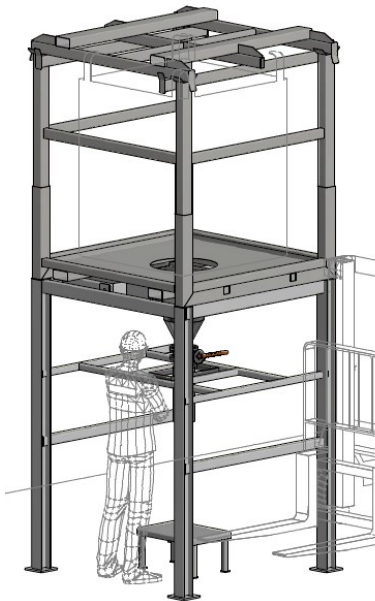
Special Design / Fork Lift Big Bag Repacking Station
