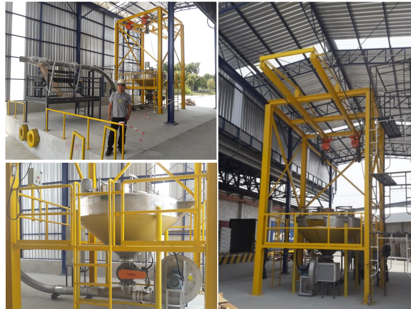
Special Design / with 2 Monorail Hoist and Extra large buffer hopper of 4,000 liter
